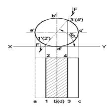
**25.** Draw the front view and top view of an equilateral triangular prism of base side 30mm and height 60 mm kept in the horizontal position, with the axis parallel to both H.P. and V.P.
