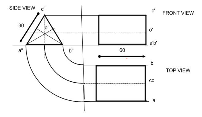
26. Project front view, side view and top view of the machine block, to scale 1:1
